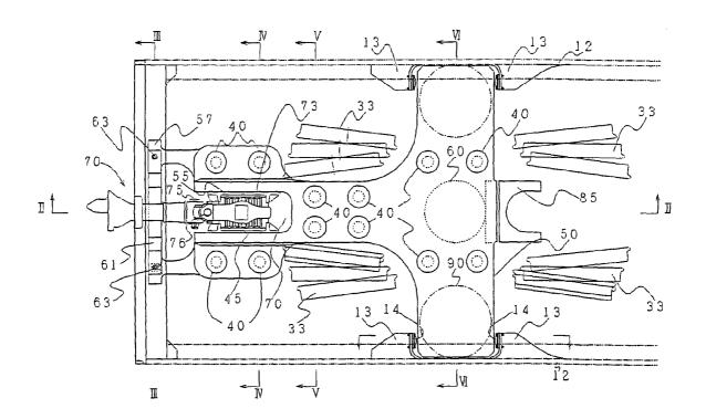
12: SIDE BEAM, 13: STOPPER, 33: WHEELS 50: SUBFRAME, 55: GUIDE, 60: CENTER PIN, 70: COUPLING ROD, 90: AIR SPRING
